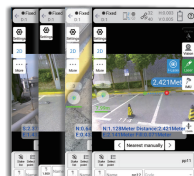
Laser Visual Survey & Stakeout
