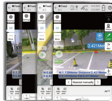
Laser Visual Survey & Stakeout
