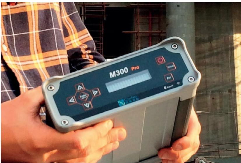
▲ Figure 3, ComNav Technology's M300 Pro GNSS CORS station.
