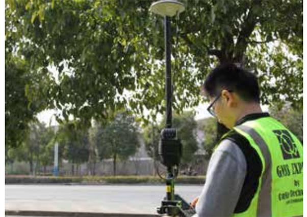
The G200 is a cost-effective GNSS receiver that provides centimeter accuracy positioning to any connected mobile devices for RTK field surveying.
