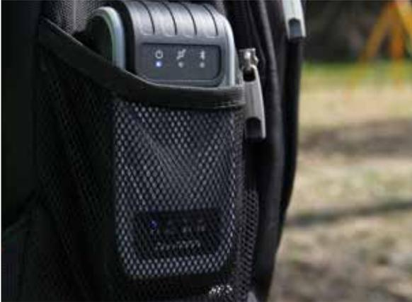
The G100 is a rugged, compact, wearable GIS receiver that provides sub-meter accuracy positioning.
